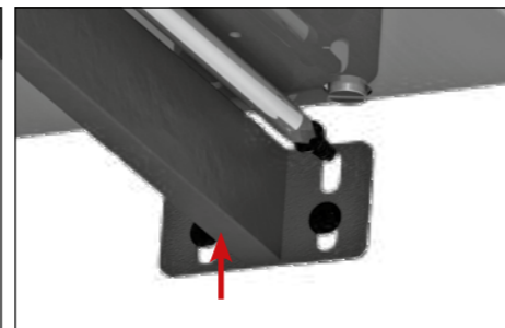
6. Push the support bar firmly against the underside of the PITT cooking unit and first tighten the upper two screws completely and then the lower screws.
